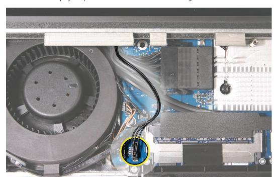
6. Connect the LVDS cable to the logic board. Replace the two T6 screws.
